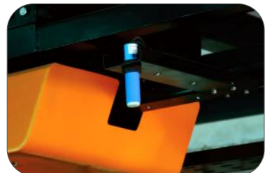
Ultrasonic sensors for Automatic vehicle length sensing
