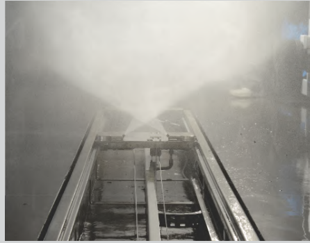
High operating pressure of 55 bar for effective cleaning
