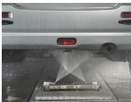
with Optional integrated UNDER CHASSIS WASHER
