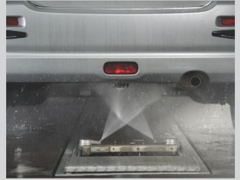
Rotating dual nozzle for better reach
